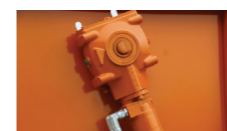
Low maintenance high torque gearboxes are used on the floor and elevator drives for reliable power transmission.
