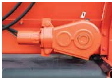
Low-maintenance, high-torque gearboxes are used on the floor and elevator drives for reliable power transmission
