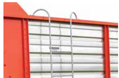
The galvanised ladder provides access to reach over the sides for adding minerals or supplements to the load
