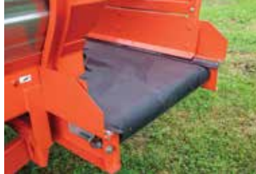
The heavy duty 900mm wide rubber belt will handle all feed products. Feed placement is controlled with adjustable belt speed
