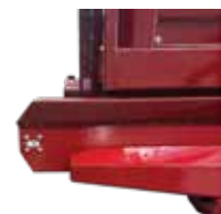
Autoshift ram extends the conveyor 200mm
