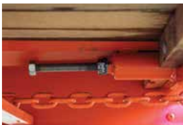
Floor and elevator chains are easily tensioned with stainless steel chain adjusters that won't corrode and seize
