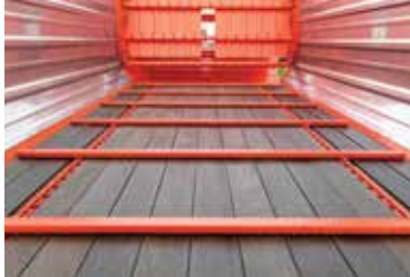
The durable hardwood floor and stainless steel sides protect against the corrosive effects of silage
