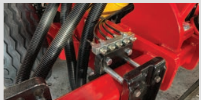
Grease bank kit - Makes greasing the hard to access grease nipples easy
