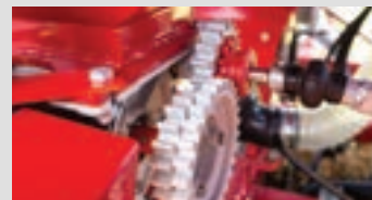
Metering distribution unit - high and low ratio settings
