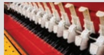
Peg seeder units with large and small seed wheels for most varieties of seed and fertiliser
