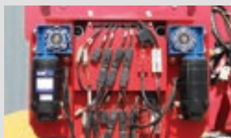
Mechanical gearboxes or high torque DC motor drives are easily adjustable and have infinitely variable sowing rate control
