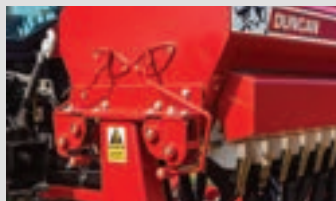
Adjustable flaps control the outlet flow
