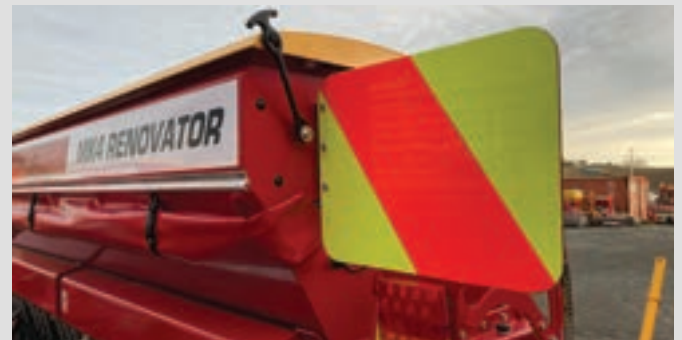
Transport visibility kit - Lights and high visibility boards for driving on the road
