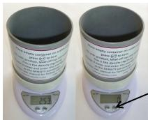
Place empty cup on scale and then zero scale by pressing button marked (७/T)
