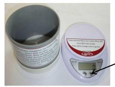
Turn scale on by pressing and holding button marked (b/T)
