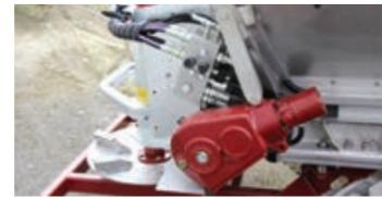
The belt is hydraulically driven through a reduction gearbox
