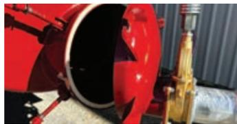
Over-centre latches on the hatches make tank access for cleaning and servicing quick and easy
