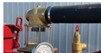
Dual brass high-flow vacuum breaker valves protect the tank and pump from high vacuum loads
