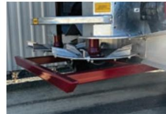
Spinner impact guard - reduces damage to spinners when operating in undulating areas or reversing
