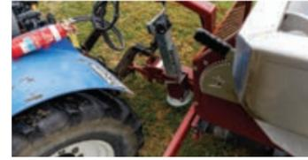
The drawbar and axle positioning is designed for a tight turning circle in headlands and optimal trailer tracking
