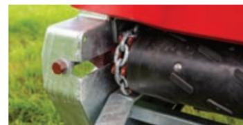
The wide rubber belt is fastened to a galvanised high-tensile chain and slat system for positive drive and no slippage
