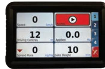
Manage and monitor all rates, spreading parameters and job records with the electronic touch screen controller
