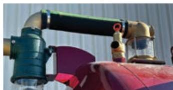
The double moisture trap system keeps liquid out of the vacuum pump to extend the service life
