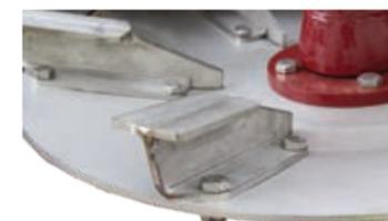
Bi-directional spinner vanes can be fitted to run the spinner discs in reverse for spreading high volume rates of lime, compost and poultry manure
