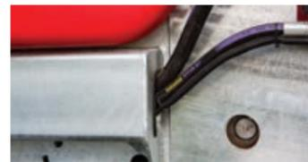
Hydraulic hoses and wiring are channelled through the chassis where possible for protection from external elements
