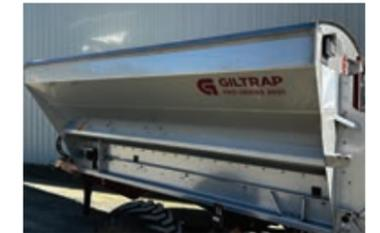
The 3mm grade 304 stainless steel bin provides years of corrosion-free use. The wide low profile bin is easy to fill and stable on steep hills
