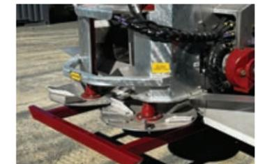
Independently touch screen adjusted spinners from the tractor seat with sectional boundary control spreading function
