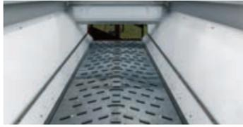
The main belt is 780mm wide with moulded cleats to handle all types of high analysis fertilisers and bulky organic products
