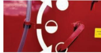
A float level indicator visible from the tractor seat shows how full the tank is
