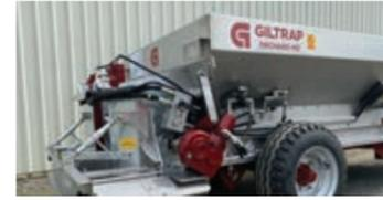
Rear banding attachments for the spinners are a great option for band spreading granular fertiliser
