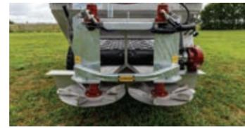
Rear mounted stainless steel spinners are bi-directional to suit the spreading application
