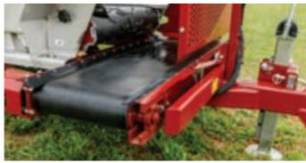
The front conveyor has a large door for high volumes. The belt is speed controlled for accurate placement
