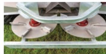
A galvanised spinner frame, nudge bar and stainless steel spinner discs enhances the WideTrac's protection against fertiliser corrosion
