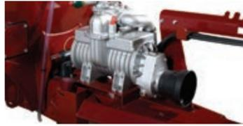
Italian Battioni Pagani rotary vane vacuum pumps are standard equipment, featuring rugged design, high airflow capacity and low maintenance requirements
