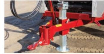
The quick lift jack and adjustable height towing eye make it easy to set the spreader up on any tractor
