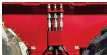
Centralised remote greasing for the axle pivot bushes makes maintenance easy
