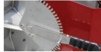
The rear door can be quickly adjusted for different rates
