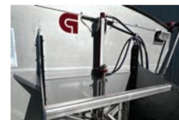
The door height is quickly and easily adjusted hydraulically with multiple spreading positions to cover the range of products and application rates
