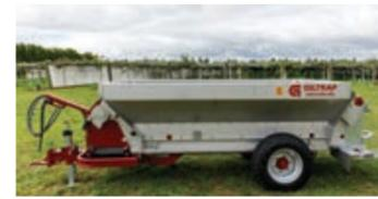
The 2.35 cu.m bin is made from grade 304 stainless steel for superior corrosion resistance
