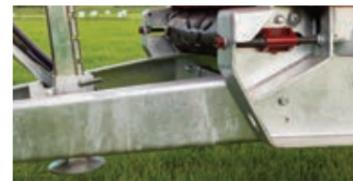
A fully galvanised chassis and drawbar on the WideTrac gives superior protection against corrosion
