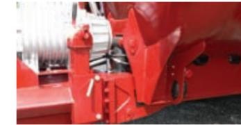
Hydraulic drawbar suspension kit - improves ride comfort and can be used to increase or decrease the tank drainage angle
