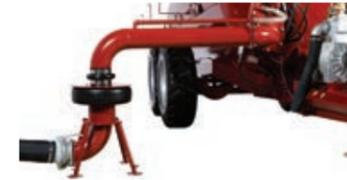
Auto-fill system with pump actuation simplifies and speeds up the filling process
