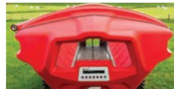
A large perspex window gives good visibility of the load and the rear gate
