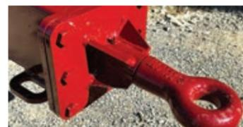
The towing connection is standard with a heavy duty swivel coupling, or can be swapped to a K80 ball hitch
