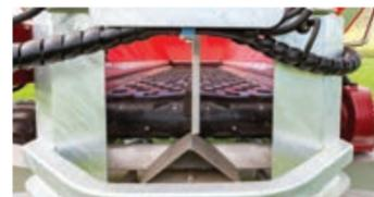
The 780mm wide rubber belt is 8mm thick, with aggressive chevron cleats to deliver product through the rear door without bridging
