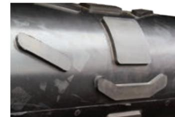
The extremely durable 850mm wide x 8mm thick vulcanised endless rubber belt, with 5mm chevron cleats, capably moves fertiliser, lime, compost and chicken manure efficiently through the rear door
