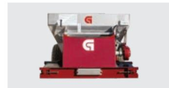
Double belt with delivery to both sides, or single belt with delivery to right hand side (see page 23)
