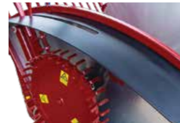
A polyethylene guard is fitted to ensure feed does not get caught in the chains or the drive mechanism
