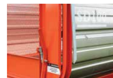
Spring-loaded trip on rear door catch
