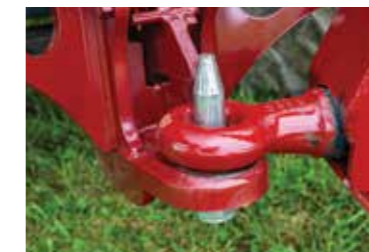
Interchangeable tow pin - can be Cat 2 or 3
