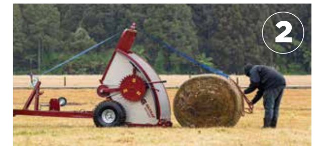
Release the winch and tilt the cradle onto the ground. Attach the two bale hooks to the winch stop. Using the hooks pull the stop out and over the back of the bale and push the hooks into the lower part of the bale
