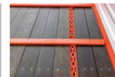
Full width floor slats ensure each load is fully cleaned out to minimise wastage. Slats are mounted to high-tensile calibrated link chain which has been proven for years in the gritty acidic silage environment, without rusting and seizing like roller chains
