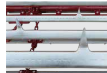
The teeth on the bars are offset to ensure even feedout of the bale. They are also tapered to release the feed easily
