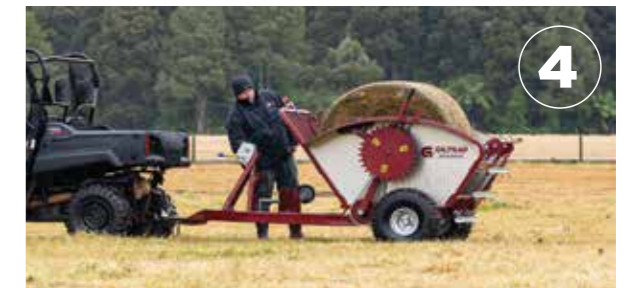
When you get to the paddock you want to feed out in, engage the ground wheel drive and you are read to go feeding. The bale will gently unroll over the back of the Bale Buggy at a ratio of 3:1 slower than your ground speed
