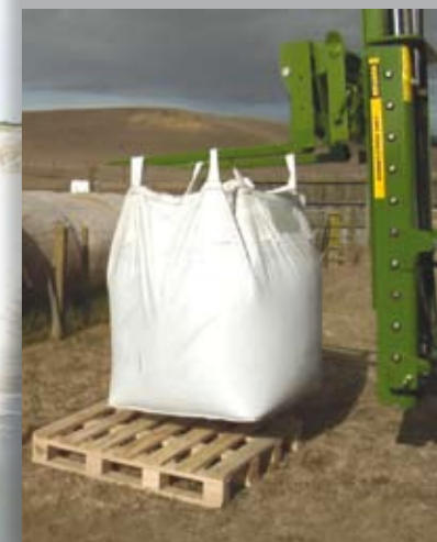
Lifting through the loops
